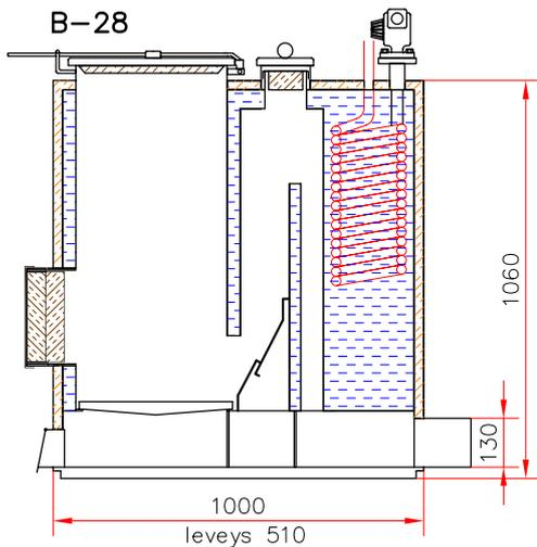
Veto B-28 boiler is equipped with a DHW water coil and a mixing valve, which enable also direct heating without a water accumulator tank. The recommended accumulator tank size is 500-1500 litres. B-28 boiler is also available with an acid-resistant fire tray. The recommended chimney height is approximately 6 metres.
