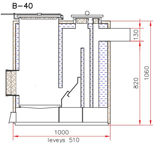
Veto B-40 is a boiler designed for use with a water accumulator tank. The small water volume guarantees efficient burning conditions and rapid heating up of the accumulator water. The recommended water accumulator tank size is 1000-2500 litres. The recommended chimney height is 6-8 metres.
